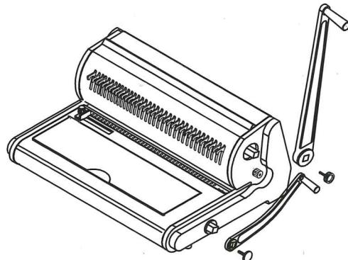
**2** Measure the thickness of paper to be bound and determine punching depth by using binding gauge. Select correct diameter of binding wire to use.
