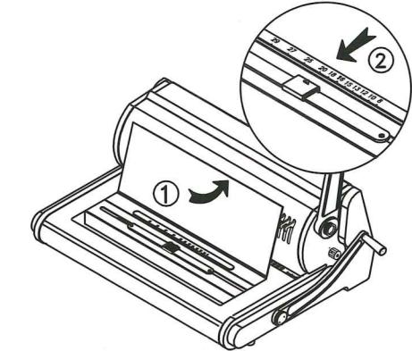
**6** 1. Remove the punched paper and insert the exposed wire fingers into the punched holes.
