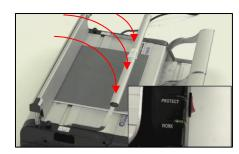
7) Carefully set the hot knife lever down and wait a few seconds until the Protect Indicator illuminates. <a href="MPORTANT!!!">IMPORTANT!!!</a> NEVER forcefully push the hot knife lever down as it may cause serious damage to the hot knife strip. Gently set it down and allow it to move along with the machine's cutting action.
