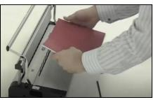
4) Position the strip on the binding channel for easier insertion of your documents.
