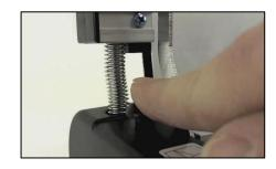
8) Set the hot knife lever to its original position then simultaneously press the paper press bar release buttons to collect your bound document.
