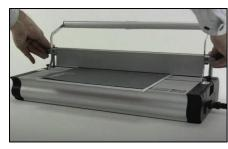
6) Set the pressure bar directly on the strip and make sure it locks firmly in place. Notice the hot knife lever's position should be exactly where it is for steps 1-6.
