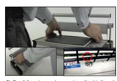
5) Carefully set your document on the binding shelf making sure the locating pin hole on the strip is properly positioned along with the locating pin on the machine.
