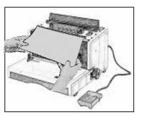
7. Gently press the coil against the inserting roller while simultaneously pressing the foot pedal.
