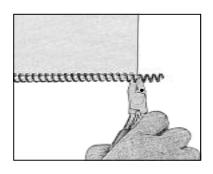
8. Crimp the ends using the handheld coil crimper pliers to keep the document from unbinding. Hold pliers as shown (red dot should be facing you.)
