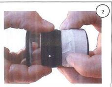
Fix the ferrule and the cylinder with scotch tape.
