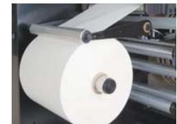
Pneumatically Activated Top-Rider Rolls for Unsupported Film and Large Diameter Rewinding
