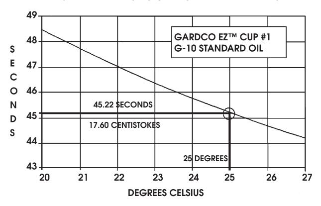
Gardco produced viscosity cups are calibrated with standard "G" Series oils. Centistoke viscosity of these oils is traceable to the National Institute of Standards and Technology. These oils are available from the Paul N. Gardner company.
