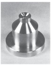
Figure 1. Standard Ford viscosity cup.
