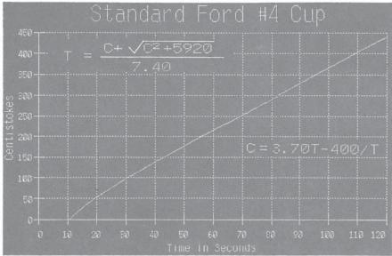
Figure 4. Standard Ford viscosity cup #4.
