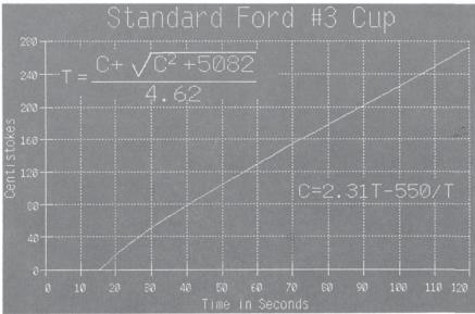
Figure 3. Standard Ford viscosity cup #3.
