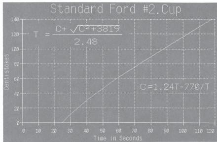
Figure 2. Standard Ford viscosity cup #2.
